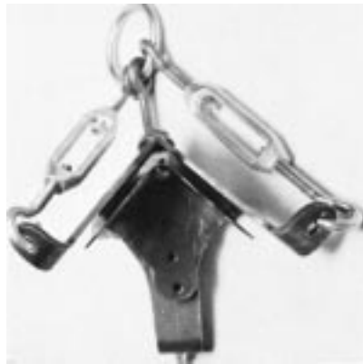
FIG. X1.4 Corner Suspension Device Attached to a Conventional Truck Corner Sealed Inside Box to Be Tested
