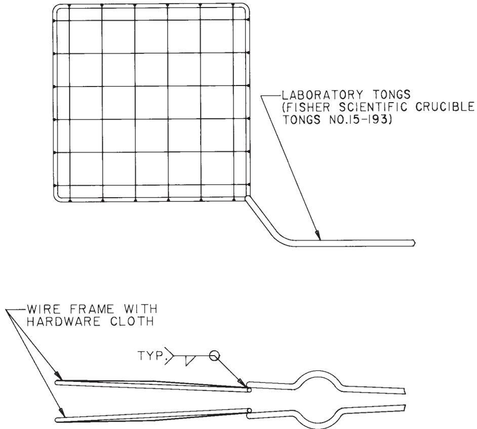
NOTE 1—Weld one wire frame to the inside of both arms of the tongs as shown.
